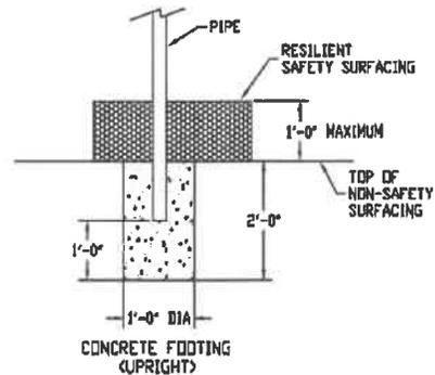
\* If resilient surfacing is to be less than 12", then additional pipe should be put in concrete to maintain proper finish grade for equipment.
