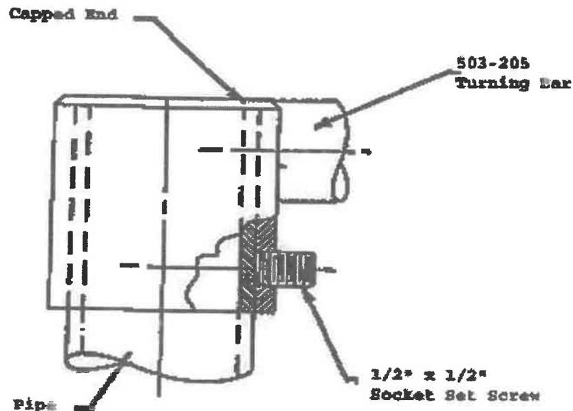
STEP #6: Plumb & level. Tighten all set screws HARD. Pour Concrete. Wait 48 hours before removing braces, installing Resilient Surfacing & using equipment.
