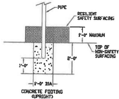
\* If resilient surfacing is to be less than 12", then additional pipe should be put in concrete to maintain proper finish grade for equipment.
