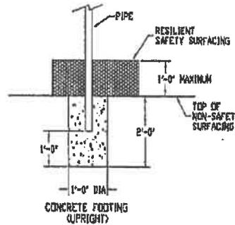
\* If resilient surfacing is to be less than 12", then additional pipe should be put in concrete to maintain proper finish grade for equipment.
